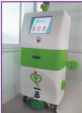
Smart Robotics Coordination System (SRoCoS) for Hospital Logistics 應用於醫院物流的智能機械人協調系統
